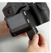
03. Insert batteries in camera
